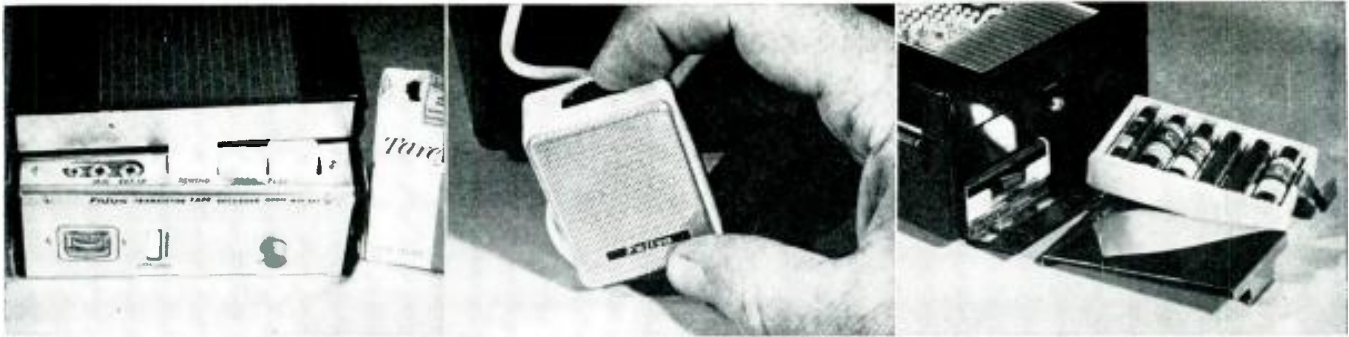
Left: All controls and jacks are on one end of the recorder. This end is up when the recorder is hung on the shoulder. The operating controls are push buttons (rewind, stop and play/record). There is also a record interlock, volume control and a meter which serves as a volume indicator and battery level check. Jacks include microphone and extension speaker. Center: Button on top of mike controls motion of recorder. Right: Penlight batteries are held in two "drawers" which are accessible through the end of the case.
