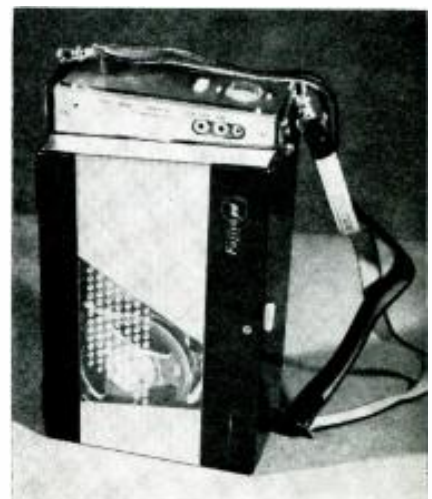
The recorder measures 9½" x 5½" x 3" and weighs four-and-a-half pounds. Controls are accessible when the case is closed.
